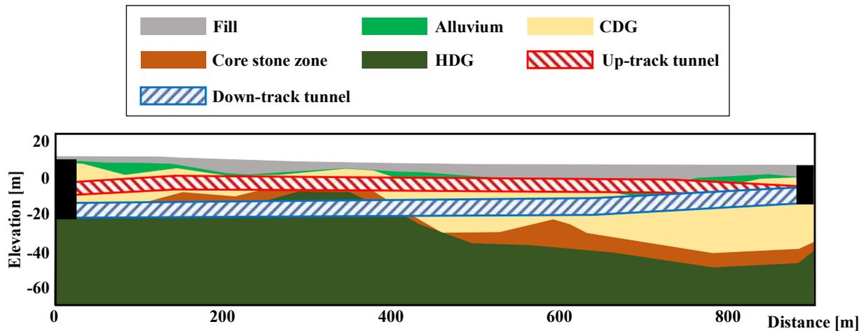
Fig. 1 Longitudinal geological profile of the site
