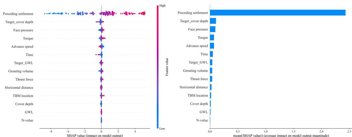
Fig. 3 Contribution of each feature on predictions of the optimal RF model
